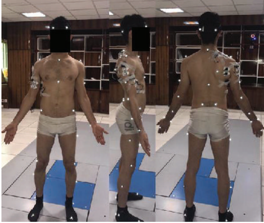
FIGURE 2: Experimental setup and 39 reflect markers and EMG electrodes were placed on the subject's bodies.
