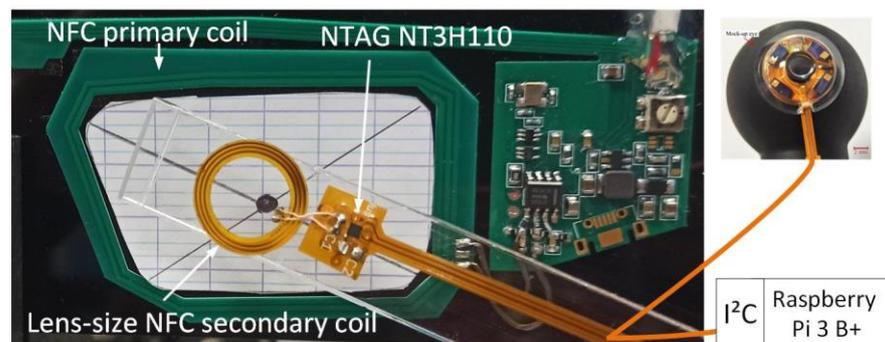
**Figure 5.** Powering the scleral lens by mean of NFC. The flexible ribbon connects the NFC chip to the encapsulated electronics to ease prototyping and the Raspberry card to retrieve the gaze direction.
