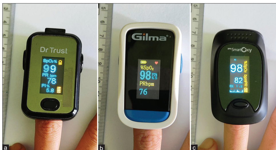
Figure 1: Three pulse oximeters – (a) Dr Trust (b) Gilma (c) BPL Smart Oxy used to measure SpO 2 . Photographs were taken when a person placed the finger in the oximeter probe without any cover
