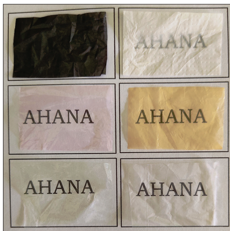
Figure 2: Sample of polyethylene plastic bags used to make finger or probe cover. From above downwards, in left column – black opaque, red translucent, green translucent; in right column – white translucent, yellow translucent, transparent. Small pieces of sample polythene bag were placed on a white paper with black bordered boxes with text
