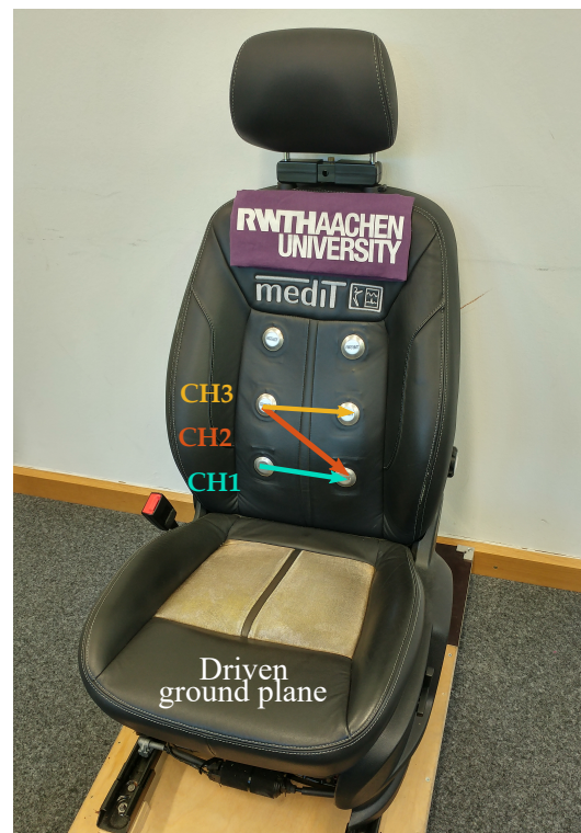
Figure 1. Positions of the capacitive electrocardiogram (ECG) electrodes on the car seat. In the sitting place, the sewn conductive textile was used as a driven ground plane feeding the common-mode signal back to the subject's body.
