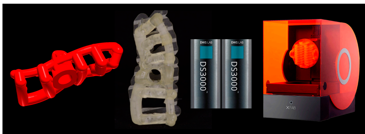
Figure 5. The open selective tooth-supported surgical template is printed with the XFAB2000 SLA printer (XFAB2000 ® , DWS, Thiene, Italy) using the DS3000 ® resin.
