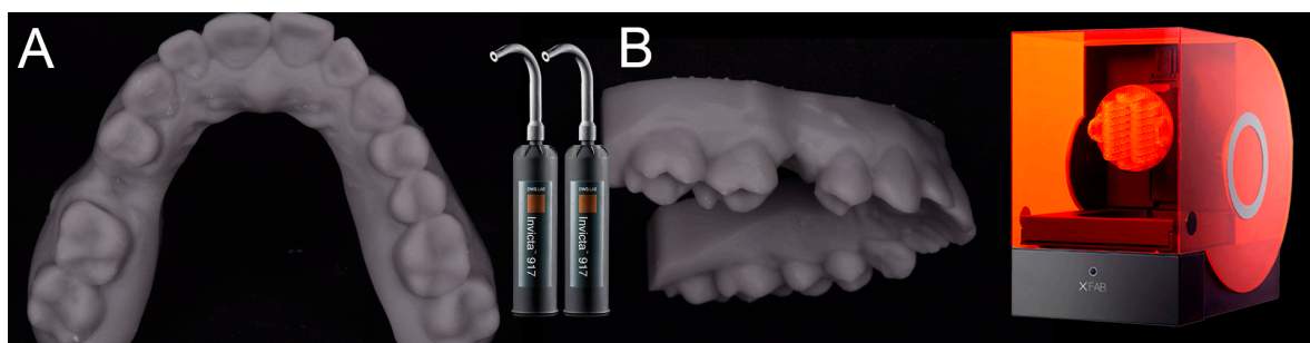
Figure 4. The models are printed in resin (Invicta917 ® ) with a desktop stereolithographic (SLA) 3D printer (XFAB2000 ® , DWS, Thiene, Italy). (A) Occlusal view. (B) Lateral view.
