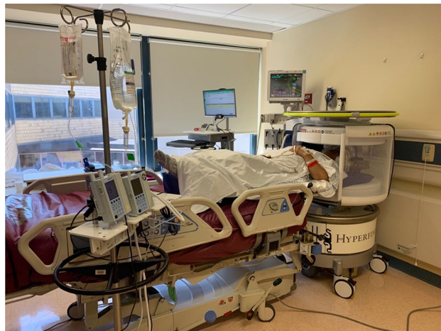
Figure 1. 0.064 T Portable MRI scanner in an intensive care unit room. Low-field portable MRI exams were performed in the presence of operational intensive care equipment. The portable MRI operator and bedside nurse were able to remain in the room during scanning. All portable MRI images were available for real-time viewing on an iPad as each sequence was acquired and processed.
