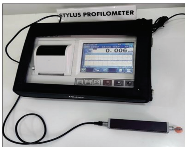
Figure 1: Representation of stylus profilometer to measure the surface roughness of soft-tissue liners
