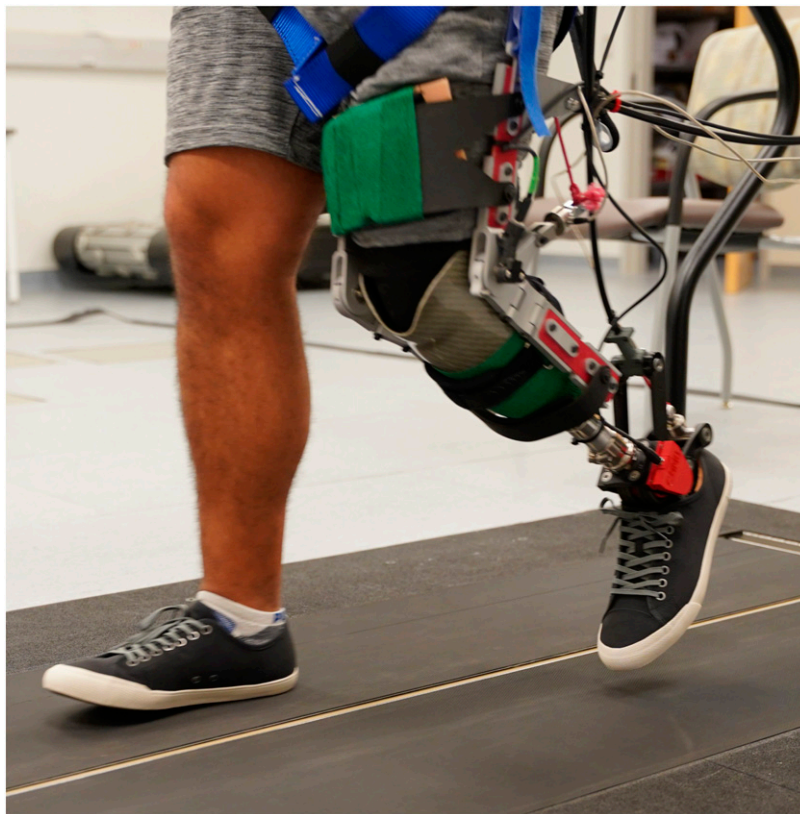
Figure 14. The participant walking with the robotic biarticular prosthesis. As the participant moves into swing phase, the knee exoskeleton cable is nearly slacked, allowing for low joint impedance during swing.
