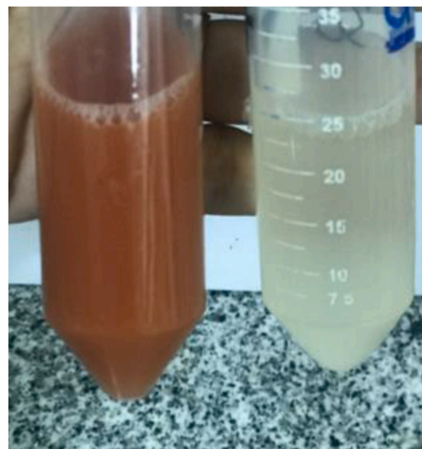
Fig. 2. Color change of the reaction solutions at different conditions; (a) Control on the right and biosynthesized SeNPs solution on left.
