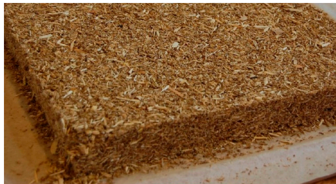
Figure 1. Particleboard matt single layered with 50% BSG after forming before hot pressing.
