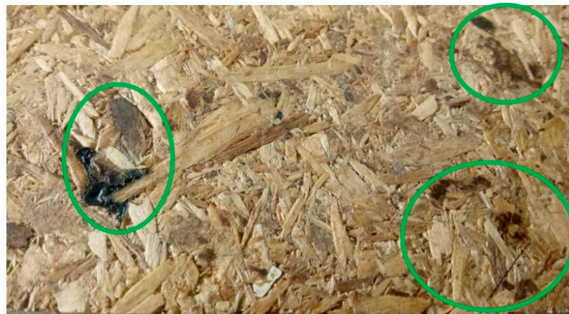
Figure 3. Dark brown spots on the surface of the panels with 50% BSG and 50% wood particles bonded with pMDI.
