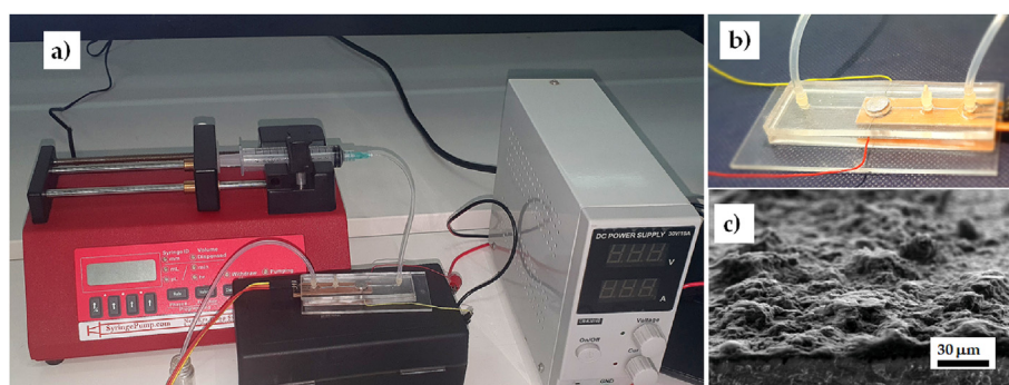
Figure 5. The setup of the microfluidic system, realized by emulating the glutamate uptake and integrated with detection: (a) the setup consisting of a syringe pump, microfluidic chip, and power supply; (b) the assembled microfluidic chip equipped with a connection pad to an electrostimulation power supply; and (c) the microstructure of the carbon matrix that resulted from the screen-printing method.
