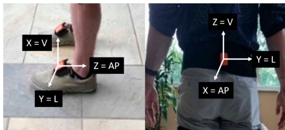
Figure 2. Sensor orientation on both the feet and pelvis. The sensor's cartesian frame matches the walking direction (L = Lateral, V = Vertical, AP = Anterior-posterior).
