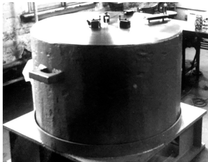
Figure 1. Steel block (1.1 m diameter, 0.76 m thickness) used for AE sensor calibration. Photograph provided by T. Watanabe of Nippon Steel Corp., Tokyo, Japan.
