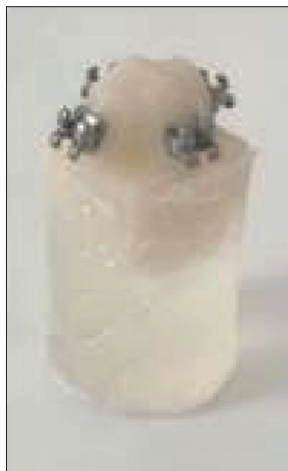
Figure 1: A customized acrylic resin block to ensure the tooth's stability
