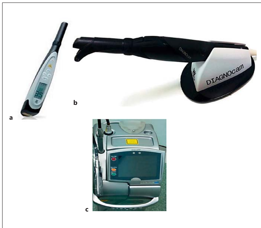
Fig. 4. Dental laser devices. a DIAGNOdent pen used for caries detection directly in the oral cavity. b DIAGNOcam used for caries detection directly in the oral cavity. c A modern laser unit (Biolase) used for soft and hard oral tissues cutting; various accessory attachments and settings can be used depending on the requirement of the clinical procedure.
