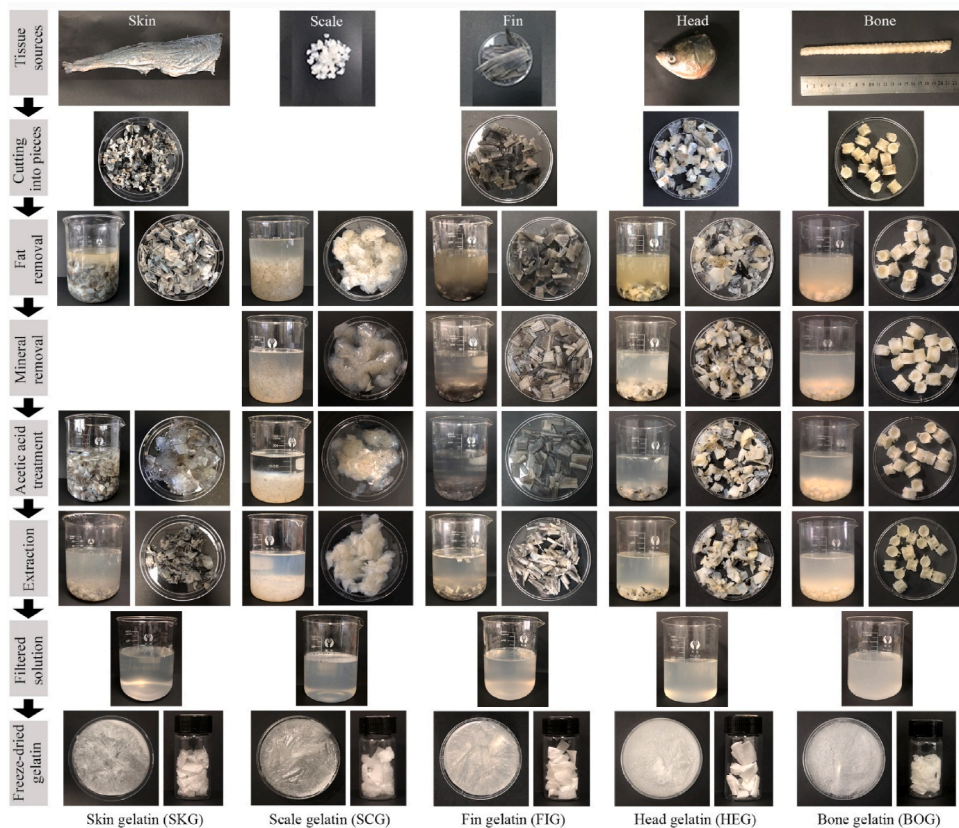
Fig. 1. Extraction process of silver carp by-product gelatins from different tissue sources (skin, scale, fin, head, and bone).
