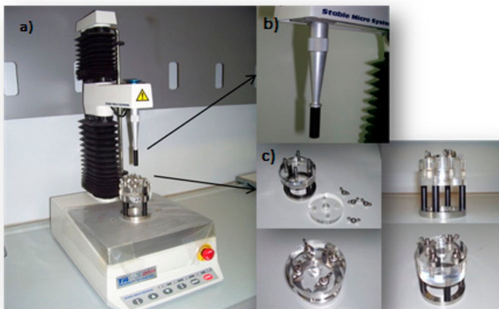
Figure 1. Scheme of the tensile tester. The texture analyzer (a) consisted of a probe (b) and a support (c).
