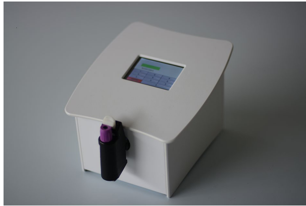
Figure 6. Point-of-care device with a EDTA collection tube (lavender cap) in the optical chamber, ready to be stirred.
