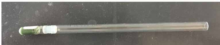
Fig. 6. picture of the sample NMR tube with its extension for introduction in the relaxometers.
