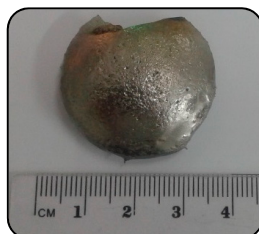
Figure 12. Exemplary cast button of HEAs.
