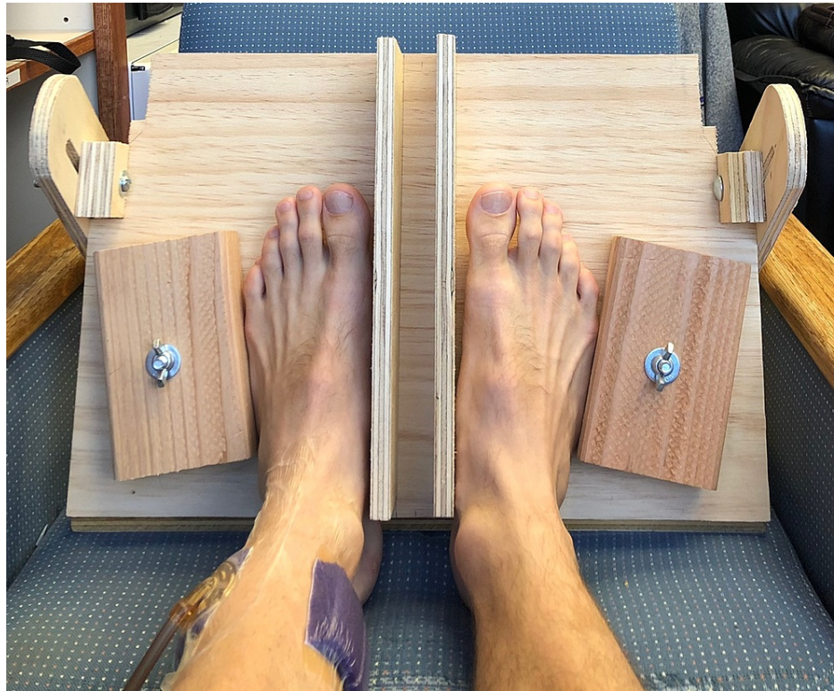
FIGURE 3: This custom jig held the feet in place to eliminate any motion artifact during the experiment. The NPWT dressing was applied to the left lower leg, proximal to the ankle.
