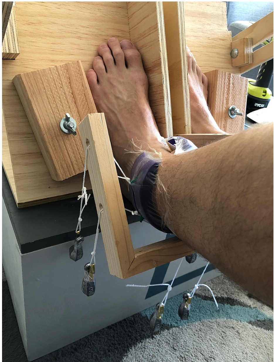
FIGURE 5: Five 85g lead weights were hooked onto loops of string that were tied onto the NPWT dressing. This provided a “lift-off” force to the dressing. Weights were used instead of negative pressure for the final experiment.
