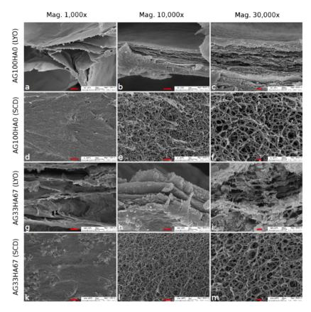
**Figure 3.** SEM images of agarose lyophilized (LYO) (**a–c**) and supercritically-dried (SCD) (**d–f**) and agarose/hydroxyapatite (33/76 w%) composite LYO (**g–i**) and SCD (**k–m**) at three different magnifications. The scale bars are 10  $\mu$ m (left), 1  $\mu$ m (middle), and 0.2  $\mu$ m (right), respectively. Reproduced from Witzler et al., 2019 [171]. Open Access Copyright Permission (Creative Commons CC BY license).
