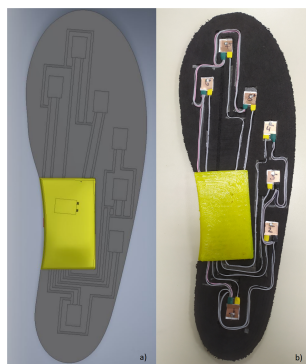
Figure 2. Arrangement of the sensors in the smart sock proposed by [22]: (a) 3D design; (b) inside view of the insole.
