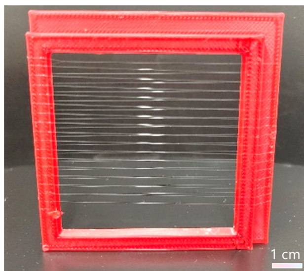
Supplementary Fig. 3. Collected PDMAEA-Q/PMAA hydrogel microfibers on a rotating frame.
