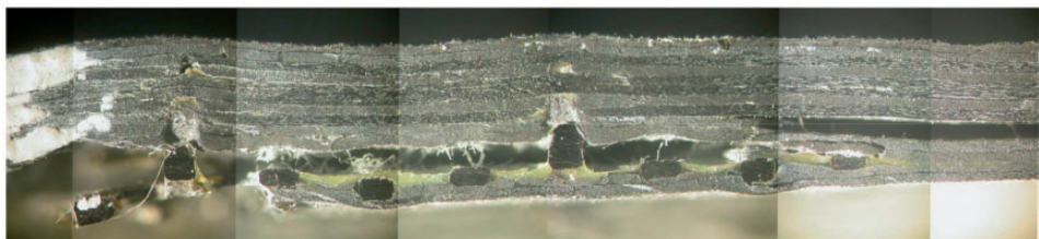
Figure 10. Photograph of specimen S1 with RHEA after the static test.
