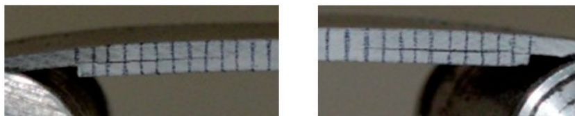
Figure 18. Zoom images of the debonding area of the co-bonded specimen B6.
