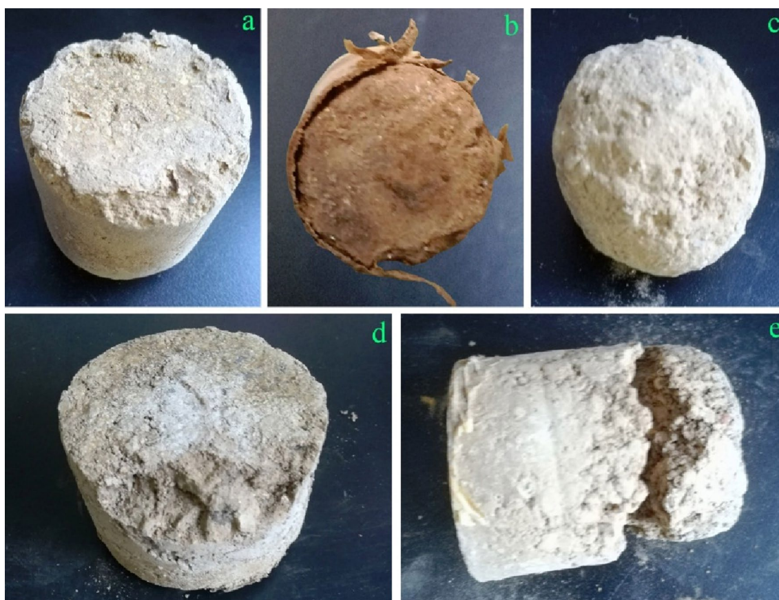
Figure 8. Typical soil column samples a–e of vertical vibration test.
