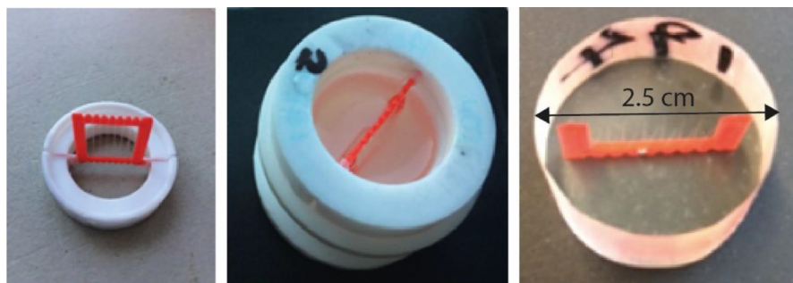
Fig. 17. Left and middle: Sample holder and mold for fiber embedding. Right: embedded fibers.
