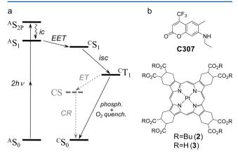
**Figure 1.** (a) State energy diagram of the processes occurring in antenna-core two-photon-enhanced phosphorescent probes. EET, excitation energy transfer; ic, internal conversion; isc, intersystem crossing; ET, electron transfer; CR, charge recombination. See text for definition of all involved states. (b) Chromophores used in construction of probe PtTCHP-C307: coumarin-307 (C307) and PtTCHP (2, 3).
