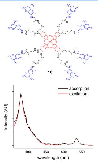
**Figure 3.** Structure and absorption and excitation spectra of model compound **10** in DMF. The excitation spectrum is recorded for the emission maximum at 647 nm.
