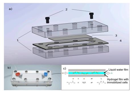
**Figure 1.** (a) Schematic presentation of a microbioreactor assembly with the main components: 1—poly(methyl methacrylate) (PMMA) plates; 2—high pressure tube fittings; 3—copolymer hydrogel layer with immobilized yeast cells; 4—non-compressible polytetrafluoroethylene (PTFE) spacer, (b) a picture of a microbioreactor between two plates with inlet and outlet fittings and (c) a schematic presentation of fumaric to L-malic acid biotransformation in the microbioreactor.
