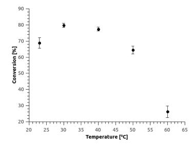
**Figure 6.** The influence of temperature on fumaric acid conversion. Inlet substrate concentration was 5 mM, while residence time was set at 30 min. The microreactor consisted of two 8/2-PBA hydrogel layers with a working volume of 350 ( $\pm$ 5)  $\mu$ L and yeast cells concentration of 188.5 ( $\pm$ 4.5) mg<sub>dw of cells</sub>/mL. Error bars indicate standard deviations of at least 3 replicates.
