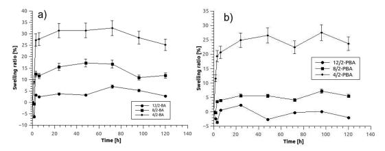
**Figure 2.** Swelling ratios of hydrogel samples of different compositions stated in legends (according to description in Table 1 crosslinked with (**a**) boric acid (BA) and (**b**) phenylboronic acid (PBA) as a function of incubation time in a demineralized water. Error bars indicate standard deviations of at least 3 replicates.
