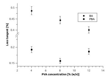
**Figure 3.** Average loss tangents of sodium alginate-polyvinyl alcohol (SA-PVA) hydrogel blends with 2% of SA, crosslinked with BA and PBA in relation to PVA concentration. Error bars indicate standard deviations of at least 3 replicates.
