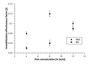
**Figure 4.** Immobilization effectiveness factor of BA and PBA hydrogel samples with 2% of SA in relation to PVA concentration. All reactions were carried at 5 mM substrate concentration, at 30 °C and at 150 rpm mixing speed. Error bars indicate standard deviations of at least 3 replicates.
