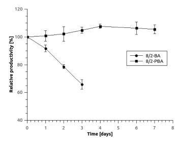
**Figure 7.** Relative productivity as a function of continuous-operation process time at room temperature. For the estimation of productivity, the flow rate of 5  $\mu$ L/min was used and the inlet substrate concentration was 5 mM. Error bars indicate standard deviations of at least 3 replicates.
