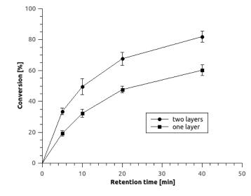
**Figure 5.** Comparison of fumaric acid conversion as a function of residence time within the microreactors using immobilized cells in one and two 8/2-PBA hydrogel layers at 30 °C and with 5 mM inlet substrate concentration at pH 7. Mean values of experimental data are presented by points with indicated standard deviations of at least 3 replicates.
