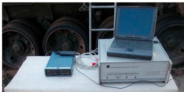
Figure 15. Measuring chain ( $\delta$ ): DMC 9012A bridge, frequency meter, laptop.
