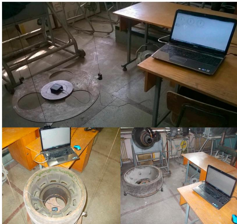
**Figure 25.** Representation of the experimental procedure for determining moments of inertia.
