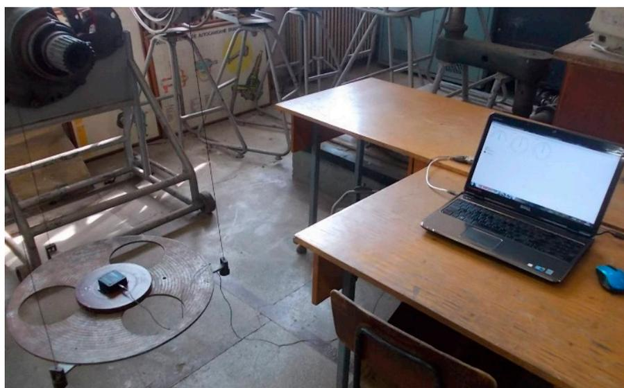
**Figure 23.** The main elements of the three-wire pendulum measuring chain.
