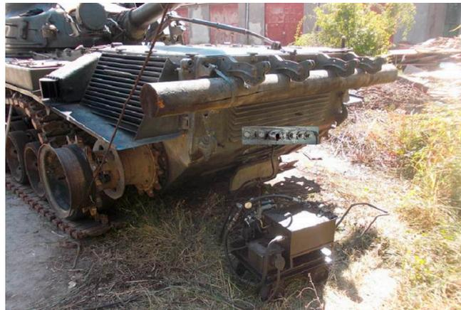
Figure 16. External gearbox coupling system.
