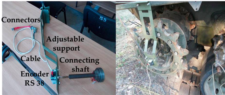
Figure 14. Mounting the RS-38 optical encoder on the right-hand drive wheel.
