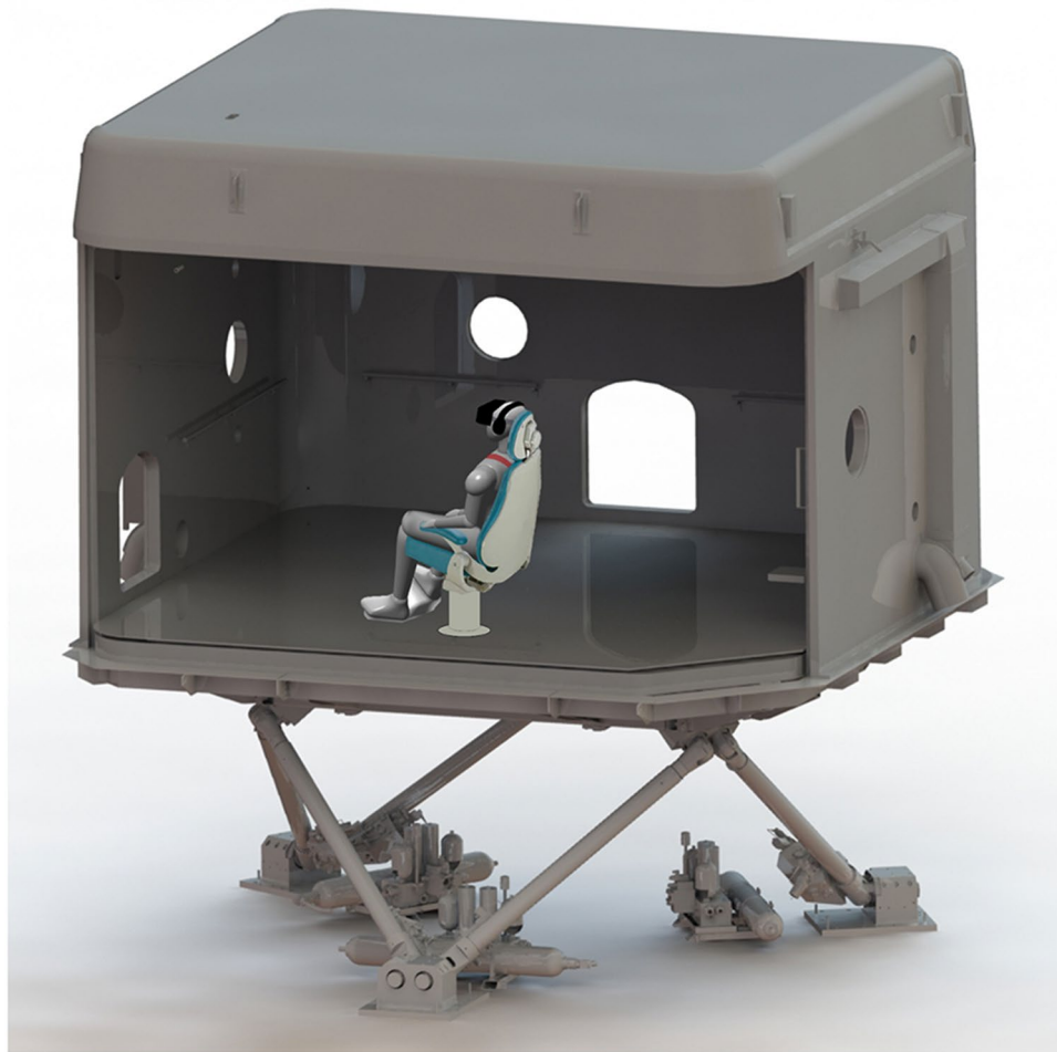
Figure 1. Vestibular psychophysics setup. Schematic of the laboratory setup for the psychophysical task including the 6-degrees-of-freedom motion platform.
