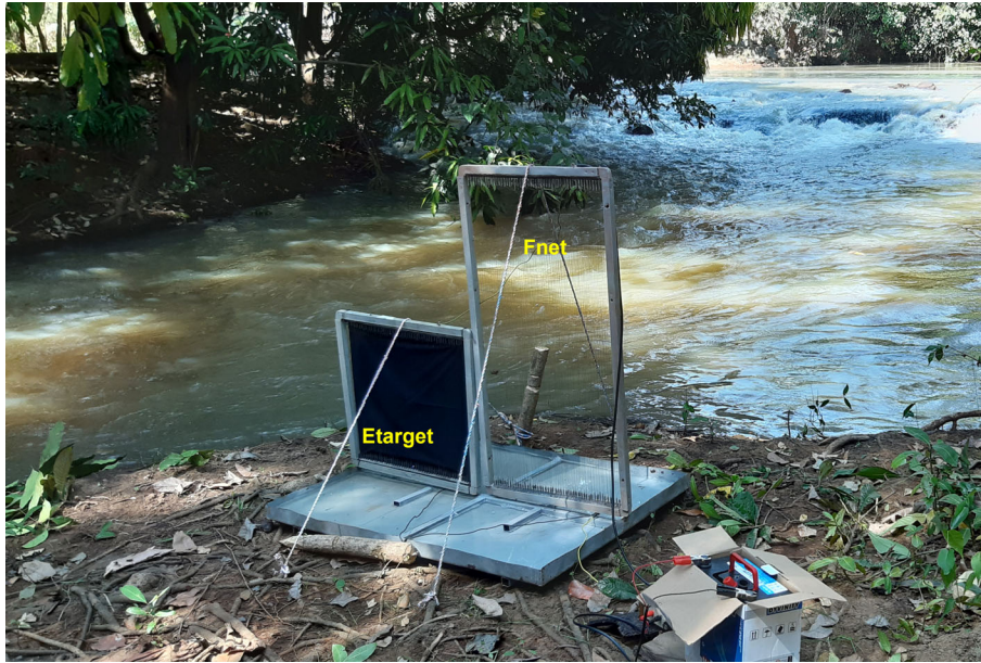
FIGURE 1 Electric grids catching devices with Etarget (grids with black cloth) at the right and flanking net (Fnet) at the right
