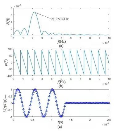
**Figure 8.** Amplitude spectrum, phase spectrum, and time-domain waveform of the gated sinusoidal driving-voltage signal. (a) Amplitude spectrum; (b) Phase spectrum; (c) Theoretically calculated time-domain waveform (solid line) and synthesized time-domain waveform (triangle-line) with the amplitude and phase spectra of the gated sinusoidal driving-voltage.
