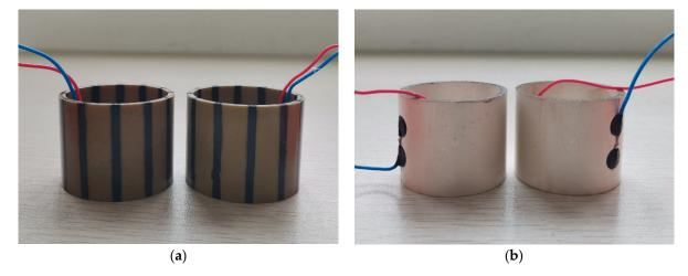
**Figure 11.** Thin cylindrical piezoelectric transducers, used in the experiments: the sides of the radially polarized thin cylindrical transducers are silvered. (**a**) Tangentially polarized thin cylindrical transducers; (**b**) Radially polarized thin cylindrical transducers.
