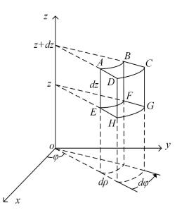
Figure 1. Schematic diagram of a microvolume element.
