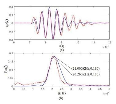
**Figure 13.** The calculated waveforms and amplitude spectrum and the experimental results used two radially polarized transducers. The solid lines are theory calculation results, and the dotted lines are experiment measurement results. (**a**) Waveforms; (**b**) amplitude spectra.
