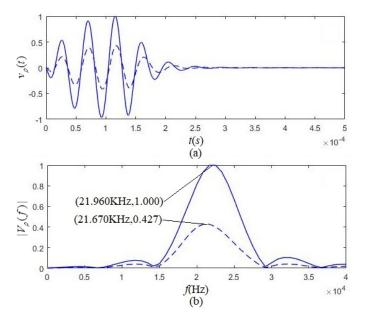
**Figure 10.** Acoustic signals radiated by tangentially polarized and radially polarized thin cylindrical transducers under the excitation of the same gated sinusoidal driving-voltage signal with the frequency of  $f_s = 22.130$  kHz, respectively. (a) Waveform; (b) Amplitude spectrum.
