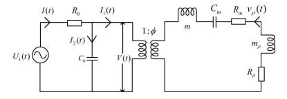
**Figure 4.** The acoustic-electric equivalent of each arc-slice of the tangentially polarized thin cylindrical transducer:  $U_1(t)$  is the driving-voltage signal that excites the source transducer; V(t) is the voltage between two electrodes of each thin arc-slice in the transducer;  $v_{\rho}(t)$  is the particle displacement velocity on the surface of the transducer;  $R_0$  is the output resistance of the driving circuit.
