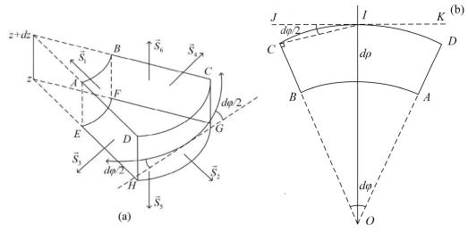
Figure 2. Schematic diagram of stresses on the microvolume element. (a) Stereogram; (b) Top view.
