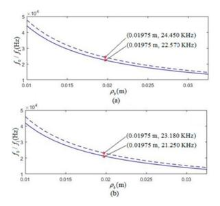
**Figure 5.** Relationship of both the free resonant frequency  $f_0$  and loading resonant frequency  $f_1$  versus its average radius  $\rho_0$  of tangentially and radially polarized thin cylindrical piezoelectric transducers. The dotted line is the case with free mechanical load, and the solid line is that with the mechanical load. (**a**) Tangentially polarized thin cylindrical piezoelectric transducer; (**b**) Radially polarized thin cylindrical piezoelectric transducer.
