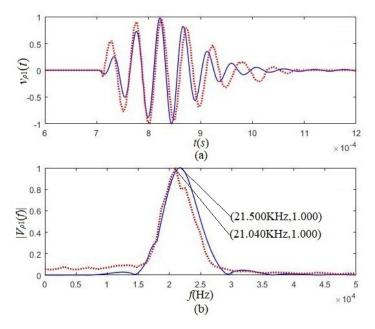
**Figure 12.** The system's calculated waveforms and amplitude spectrum and measurements consist of two tangentially polarized transducers. The solid lines are theory calculation results, and the dotted lines are experiment measurements. (**a**) Waveforms; (**b**) amplitude spectra.
