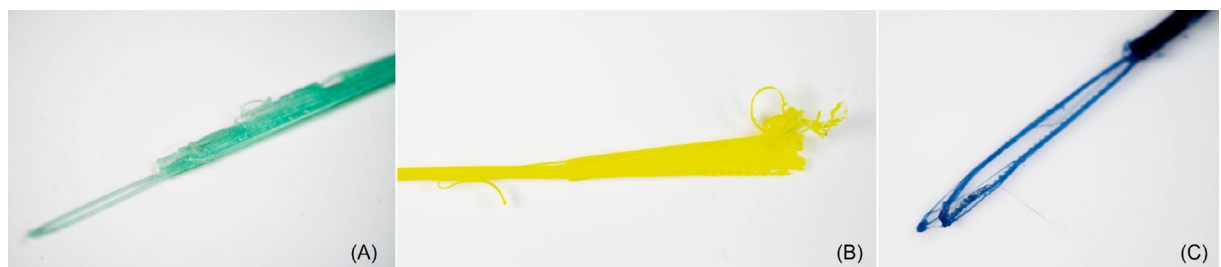
Fig. 8. Examples of fabrication failures that occurred in 3-D printing of the vitrification wands of the VD-FS, including inappropriate adhesion among layers (A), inconsistent adhesion to build plates (B), and stringing (C).
