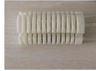
FIGURE 9: Physical model of pneumatic soft-bodied bionic actuator.
