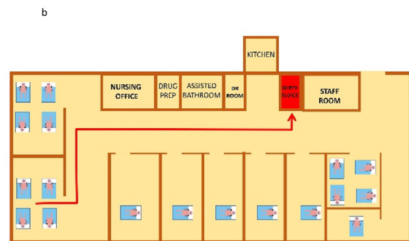
Figure 2. Layout of (a) an actual intensive therapy unit and (b) a medical ward detailing the distances staff have to travel carrying contaminated body fluids.
