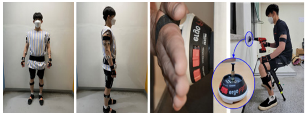
Figure 4. Motion capture system (MVN Awinda, left) and drilling force measurement system (ergo FET, right).
