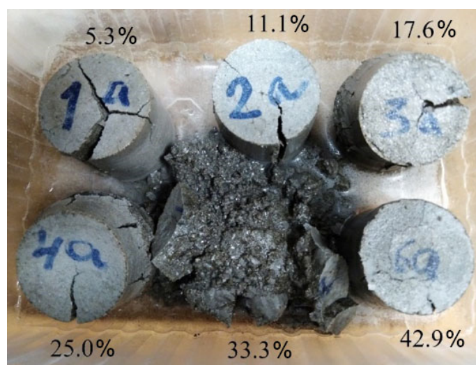
Figure 10. Expansion of specimens with content of silica fume additive from 5.3% to 42.9% by weight of fly ash after 11 days of air curing and 2 days of water curing.
