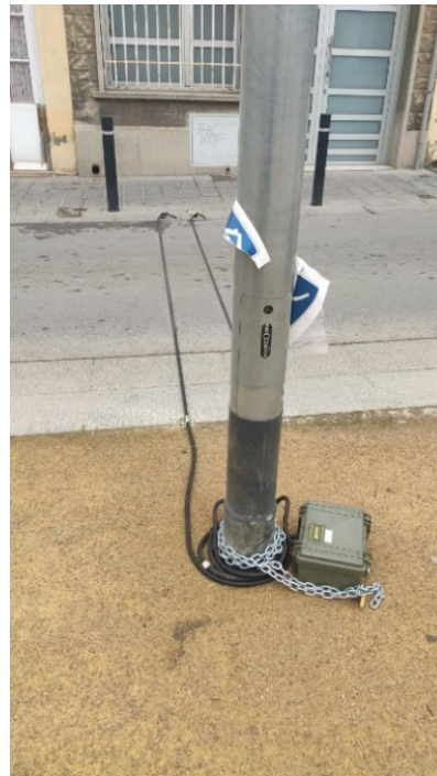
Figure 8. Circulation counting mechanical sensor (photo by author) located at M2 according to Figure 6.
