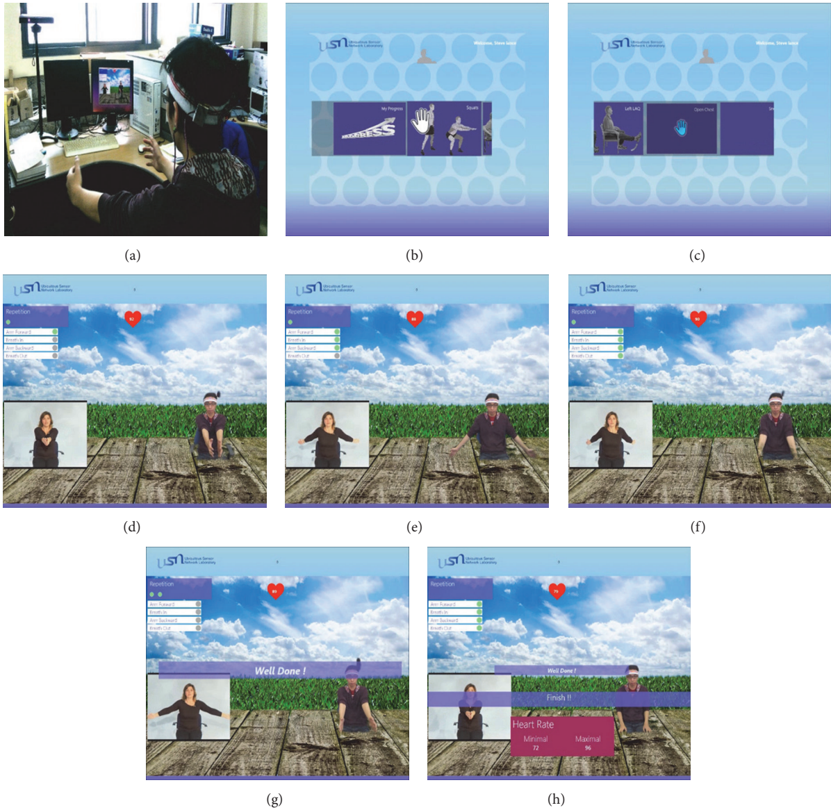
FIGURE 5: Demonstration of the proposed system: (a) user following guidelines provided by the system in real time; (b) main menu; (c) user selects exercise; (d) state one of open-chest exercise; (e) state three of open-chest exercise; (f) state four of open exercises; (g) completion of a repetition of an exercise; (h) completed set of exercises and heart rate information.
