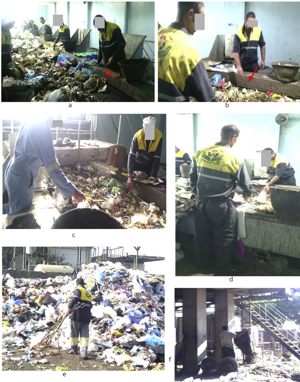
Fig. 3. Worker are not wearing proper PPE at the solid waste sorting facility in Alexandria and are performing hand picking without gloves (a-f). Red arrow in (a and b) points to a hook used by some works to pick the waste.
