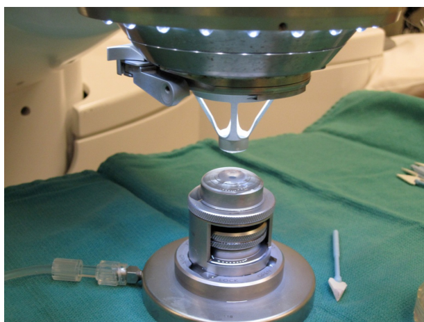
Figure 1 The setup for applanation of donor cornea with an artificial anterior chamber system and femtosecond laser cone.
