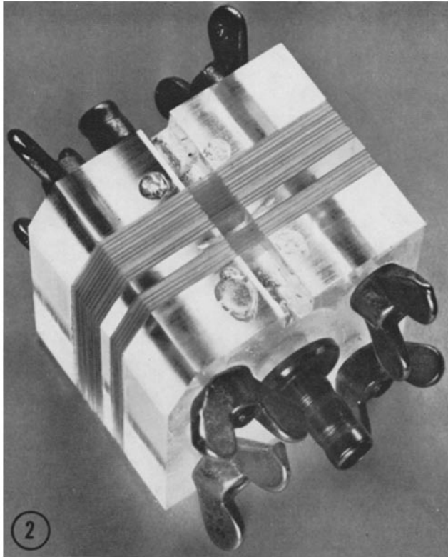
FIGURE 2 Lucite chamber with compartments allowing the recording action potentials using electrodes located on the pre- or postganglionic nerves (see Fig. 1). The central tubing allows the block to be warmed by circulating water.
