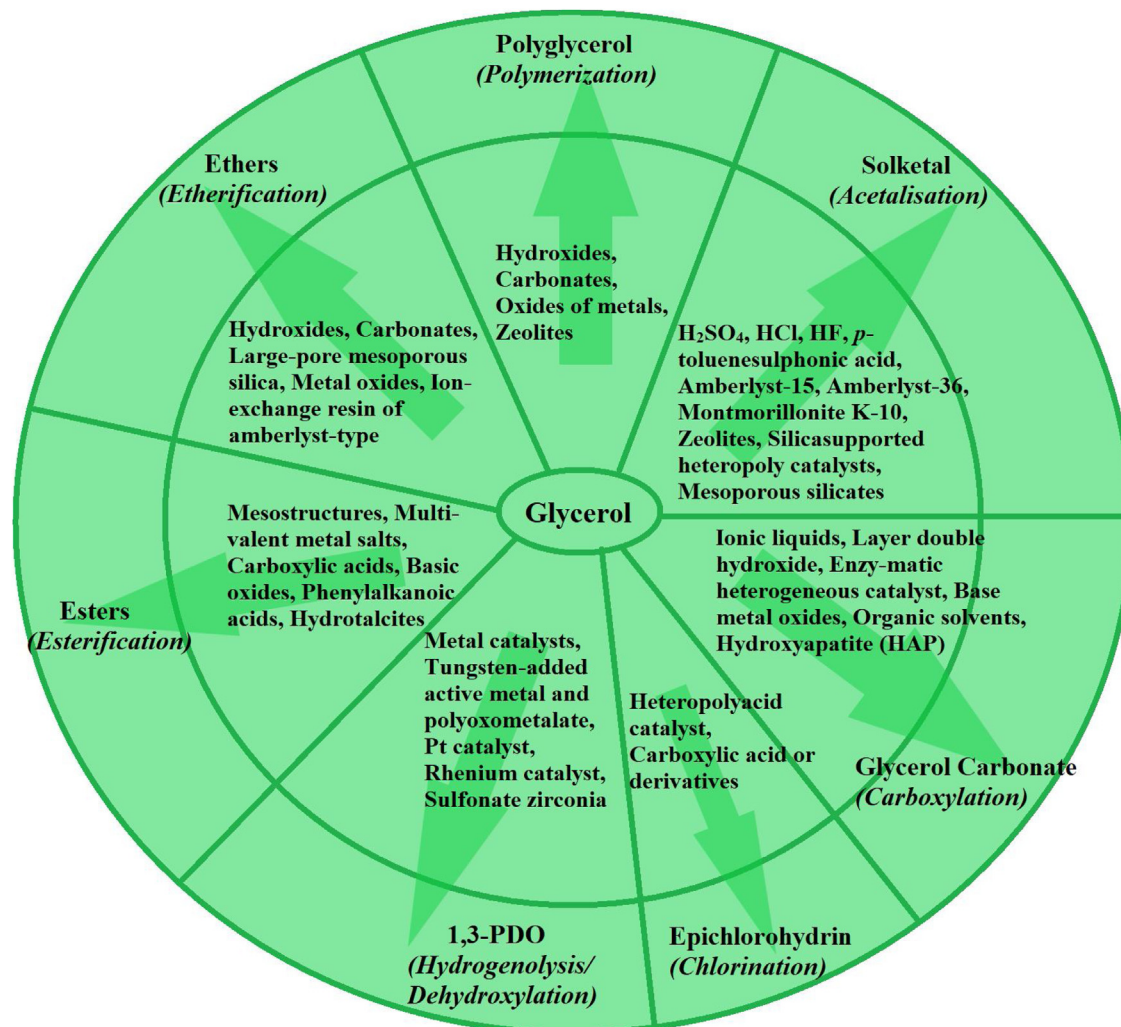
Fig. 5. Chemical reaction pathways for conversion of crude glycerol to value added products [[7,18,36,37,53–56].
