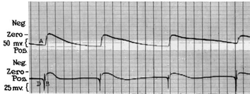
FIG. 5. Photographic record of successive variations produced by application of 0.001 M KCl saturated with chloroform at C (Fig. 5 a ) with 0.001 M KCl at A , B and D . The two strings of the double string Einthoven galvanometer were connected as shown in Fig. 5 a .
