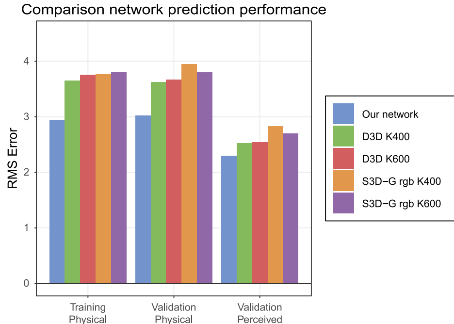
Fig 12. Viscosity prediction error for two (D3D and S3D-G) video action video classification networks. These networks were trained on two different datasets, the Kinetics 400 and Kinetics 600 datasets [31] where the numbers represent the number of classes in the dataset. For S3D-G we used the pathway that uses RGB images as input, this particular network has a pathway using optical flow input as well. As in Fig 4, we report training error using physical viscosity labels (average of last ten batches), and the validation error for both physical and perceived viscosity labels.
