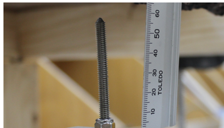
Figure 3. The penetrometer tip.
