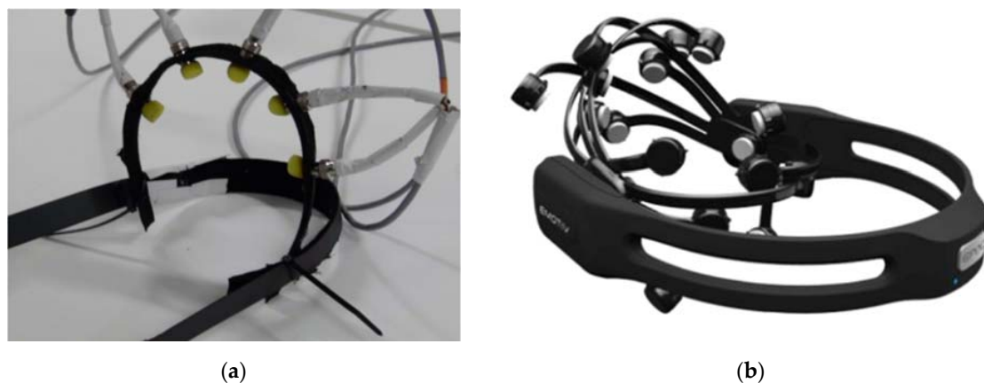
Figure 7. The used EEG headsets for this research: (a) in-house developed 5-electrodes EEG headset using the OpenEEG project; (b) the Epoc+ headset with 14 electrodes by Emotiv.
