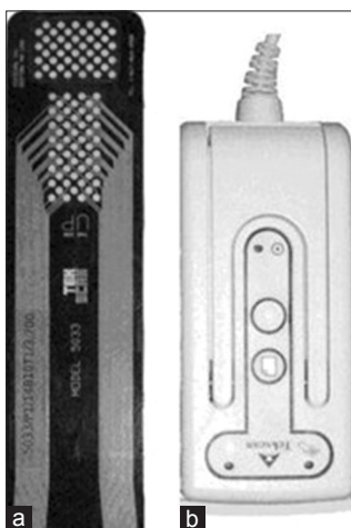
Figure 2: K-scan pressure sensor and Evolution USB Handle (Tekscan, Inc., Boston, MA). (a) Pressure Sensor (b) USB Handle
