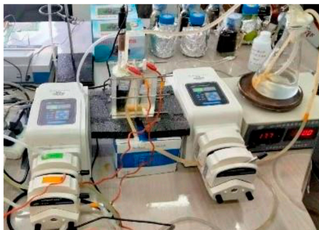
Figure 2. (A) Schematic diagram of the dual-chambered MEC. Note: A, anode chamber; D, desalination chamber; C, cathode chamber; R, resistance; and EPS, external power supply. (B) Experimental diagram of the dual-chambered MEC.
